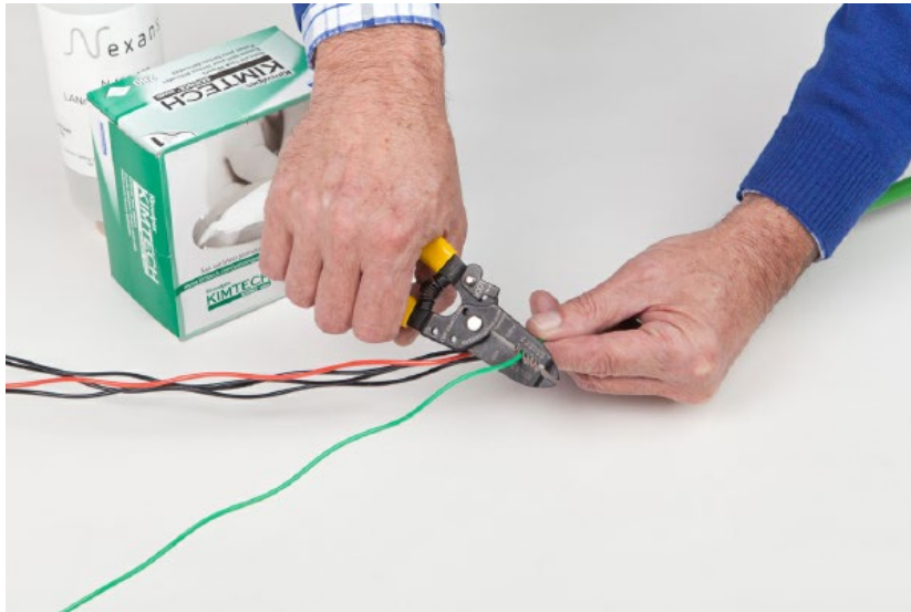
2. Cut and strip the tube
