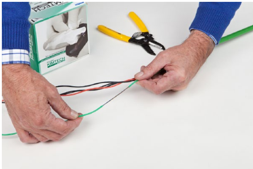
3. Remove the excess of degreaser from around the fibres
