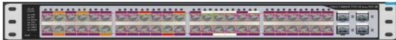
Real time graphical representation of the switch. If skilled IT staff aren't available for remote offices, visual guidance can help an unskilled person perform patching changes.
