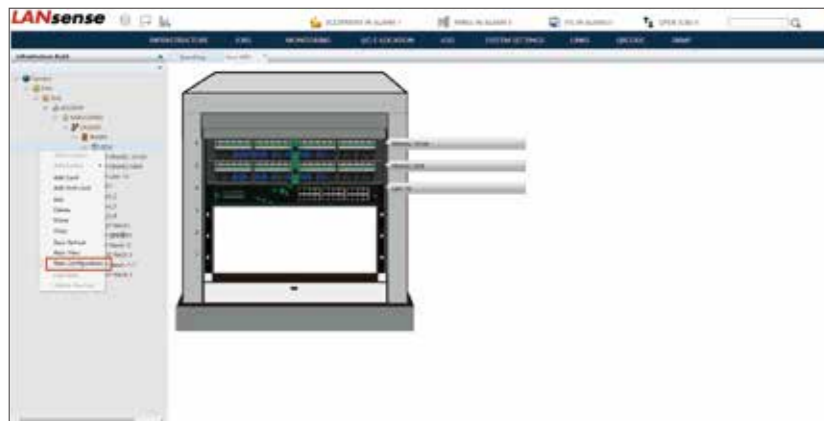
Real time 2-dimensional graphical view of equipment room, cabinets/racks, networking equipment, cabling, patch panels and LANsense TGA active equipment.
