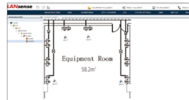
The LANsense Room Planner tool is an interactive tool for documenting the various elements and items related to cabling infrastructure like racks/floor boxes, data sockets, wall boxes, etc. Circuit tracing can also be done from the socket to find the switch port that the socket is connected to. Room plans also display available U space. The room plans of data centres, equipment rooms, can be uploaded using .svg files.
