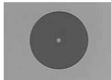
Fibre singlemode parfaite Perfect singlemode fibre
