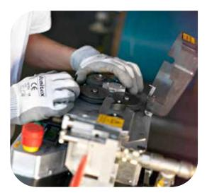
During our fibre seminars, experienced installers have shared achievements of reaching blowing distances up to 3000 meters using traditional fibre optic cables in conventional ducts. In the concluding stretches of the access network, blowing
