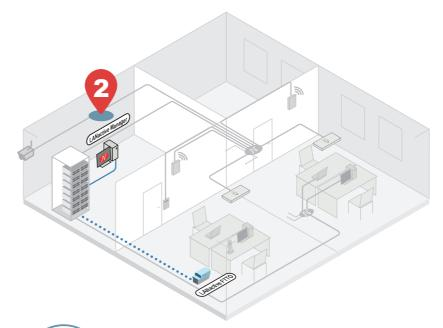
The LANactive switch starts automatically the communication with the LANactive Manager and is authenticated.
