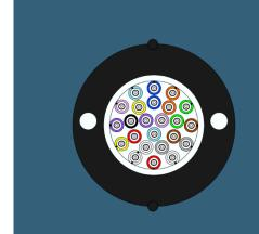
Facade distribution cable has been design to match perfectly with the walldrop façade box
